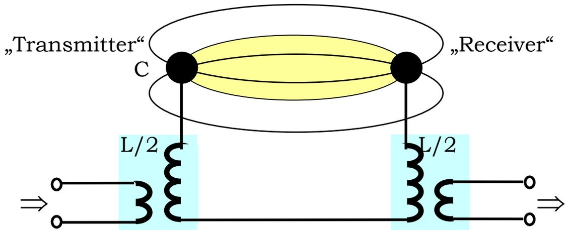
Figure 1: Interpretation as an open resonant circuit
